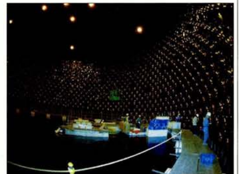
The Superkamiokande detector – taking data again after an accident destroyed over half of its photomultipliers in November 2001.
