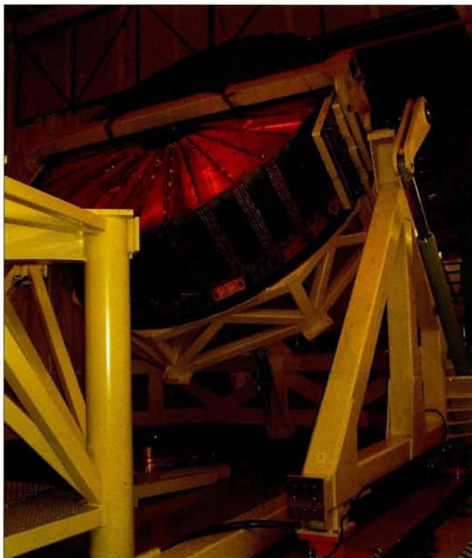
One of two HECs delivered to CERN for ATLAS.
