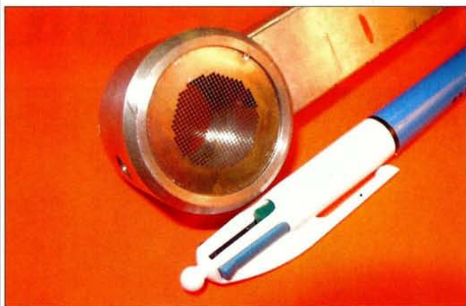
ASACUSA's microwave cavity. The fine mesh windows admit the pulsed antiproton beam on one side and the two laser beams on the other with 90% efficiency. They are, however, opaque to microwave energy introduced into the cavity through the rectangular waveguide.
