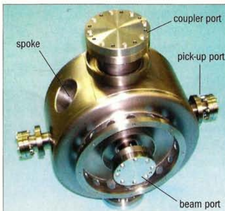
The Los Alamos spoke cavity in section (left) and assembled. The cavity's diameter is 40 cm.
